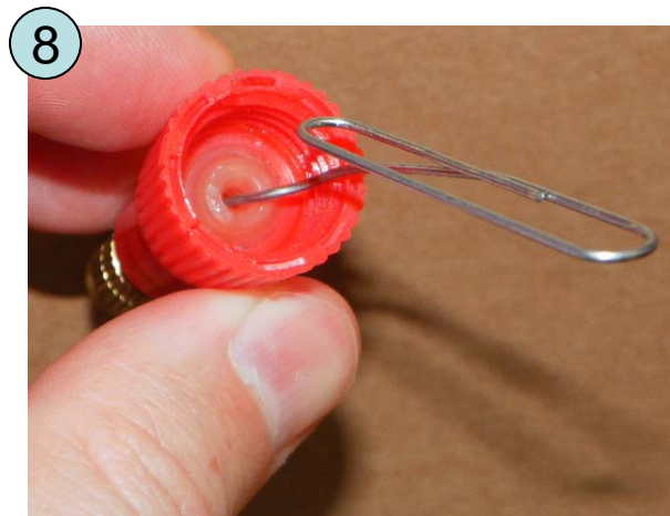
Alternate method for hardened clogs is to use a paper clip to clear the orifice.
