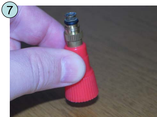
Firmly tap the end of the red nozzle extension on a table top expelling solidified product.
