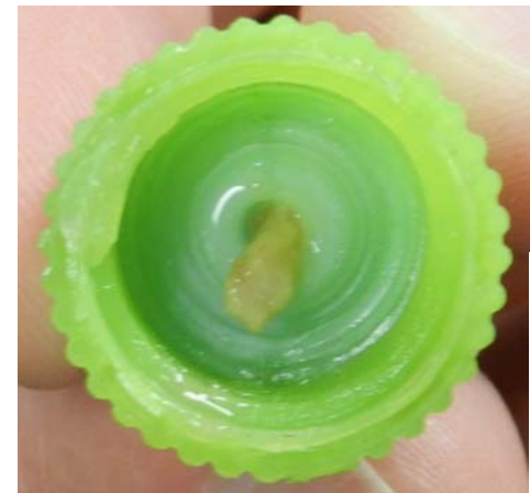
Example of clogged nozzle extension.
